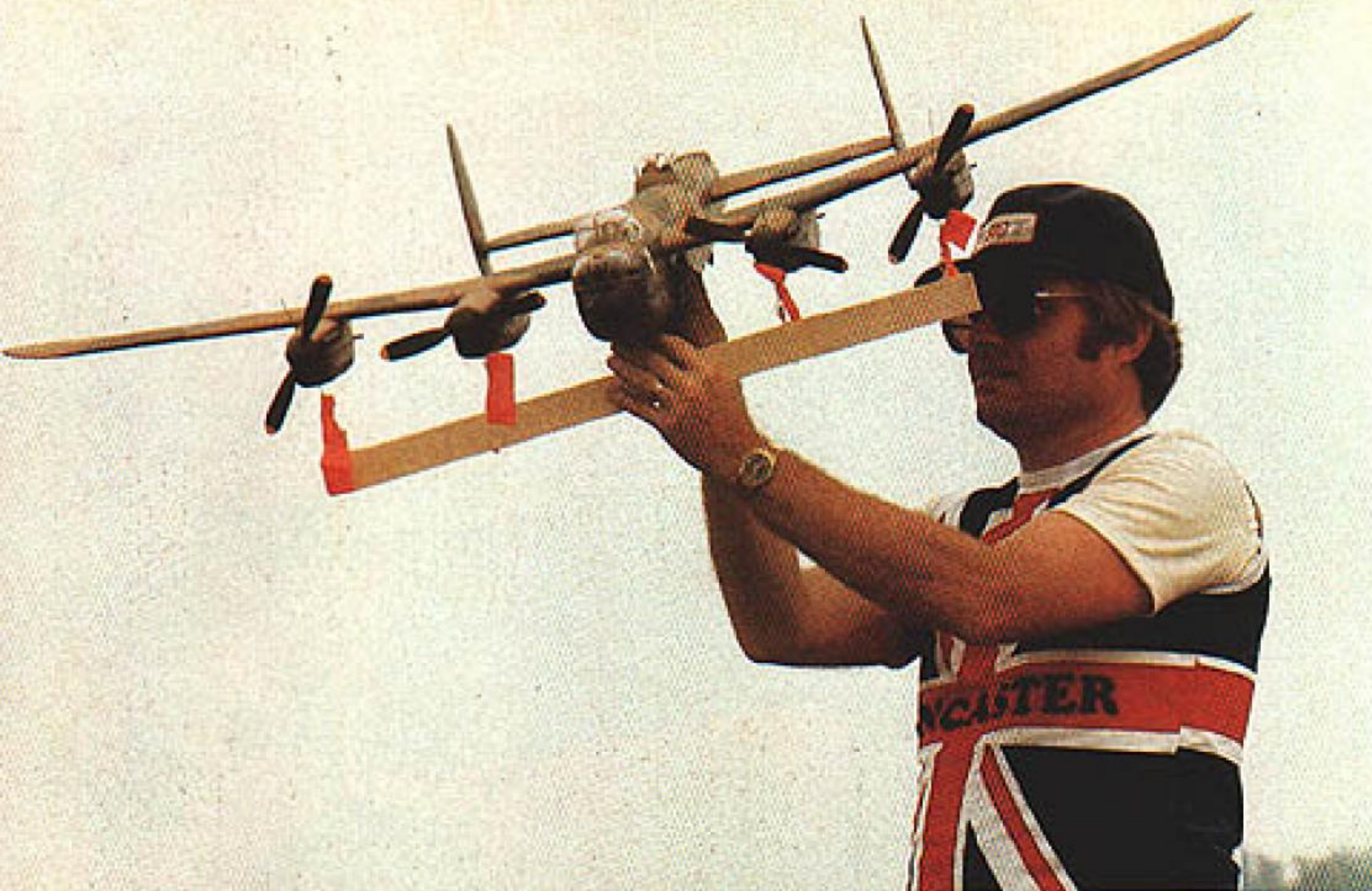
Fully wound with flagged retaining pins and pull bar in place, the Lanc is ready for another mission. Pins are inserted individually into each motor, then connected to the pull bar.
