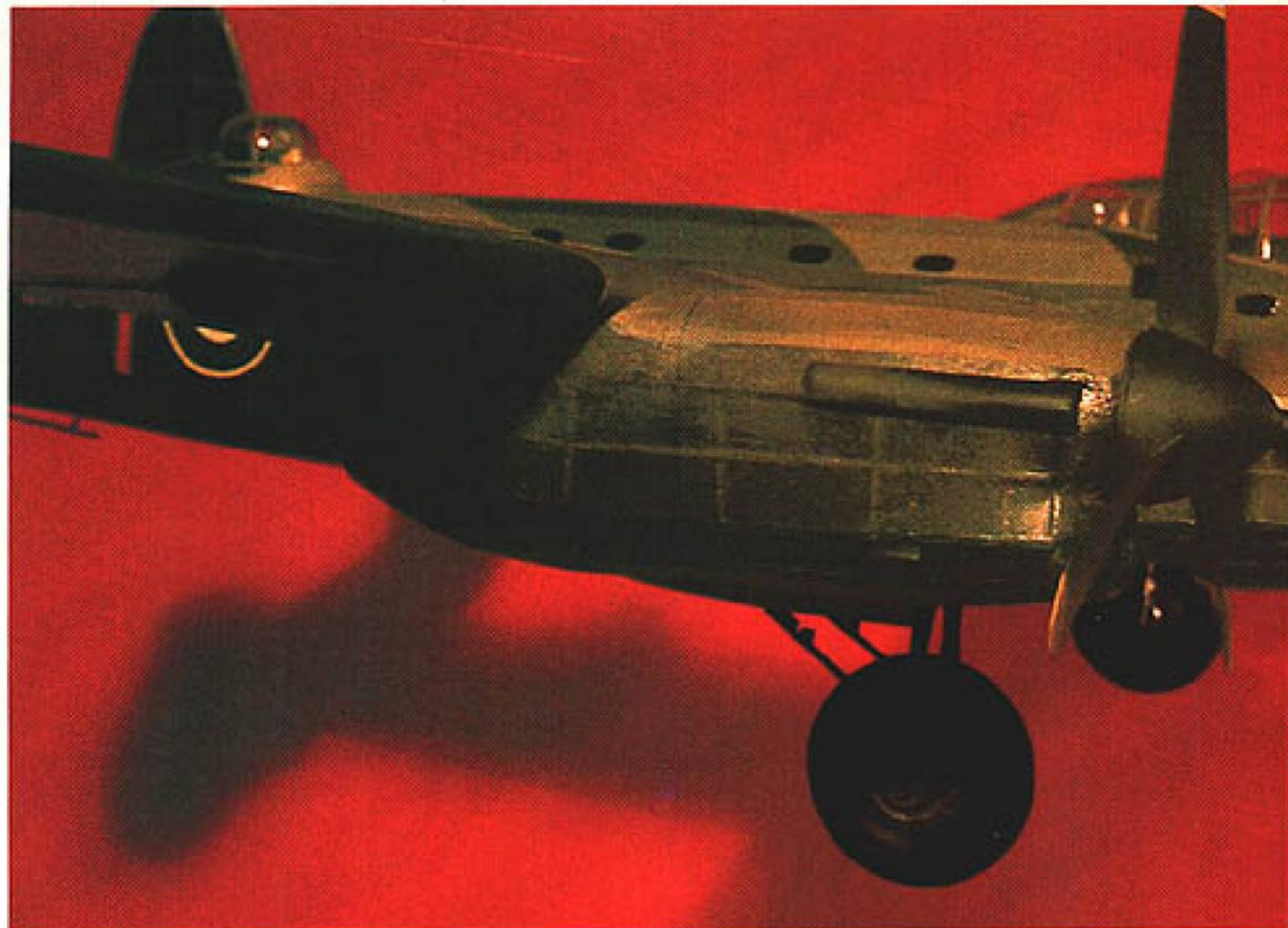
Massive yet simple, model's main gear plugs in for static display and is removed for flight. To see this model lumber up from an ROG would be a stunning sight worth lower flight times.
