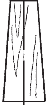
Tail Wheel Plate 1/8-inch Ply
